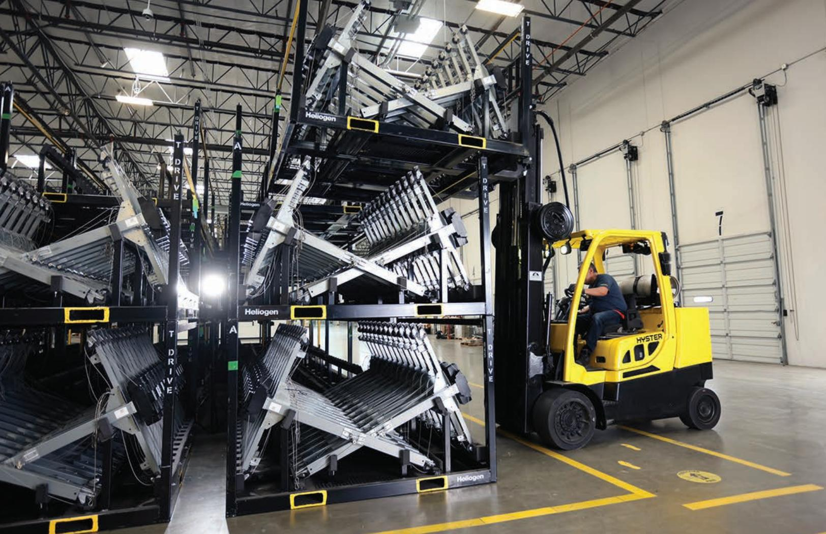
Finalized heliostat T-drives placed in reusable shipping containers
