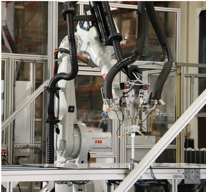
Robotic arm dispensing adhesive during mirror assembly
