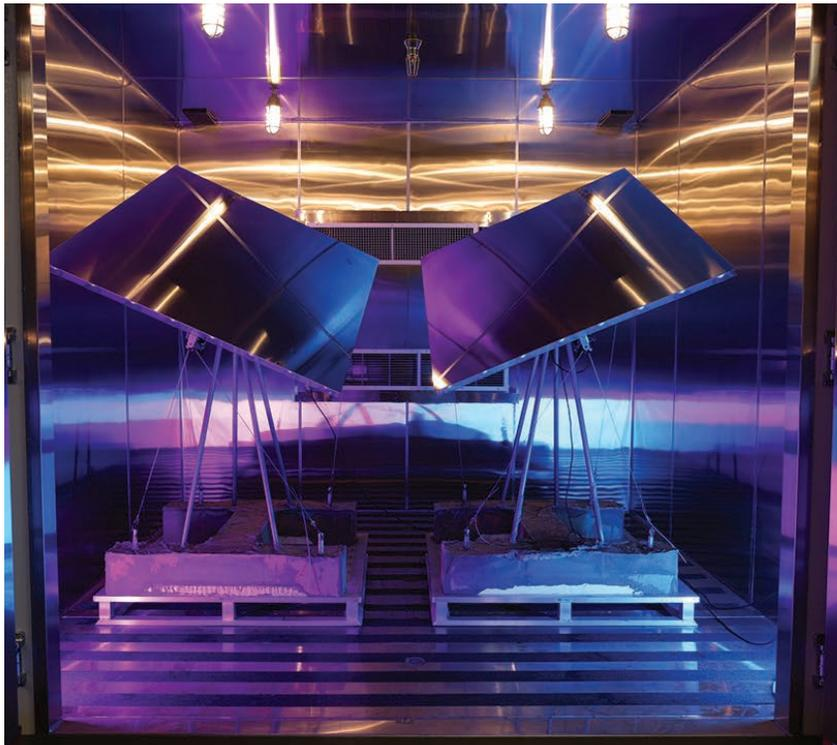
Mirrors undergoing lifetime testing in the environmental chamber
