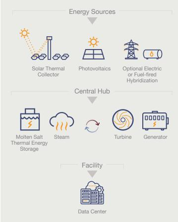
Heliogen's unique hybrid system provides a costeffective, highly reliable, carbon-free power source. Two complimentary technologies — CSP with high-capacity thermal energy storage, and PV enable data centers to tap into the power of the sun around the clock. The system maximizes and stores energy from the sun over a 24-hour cycle, overcoming intermittency while greatly reducing reliance on unstable grids.
